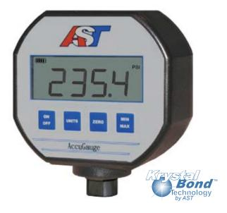
The **AG100** series is a media isolated digital pressure gauge featuring multiple measurement units, min/max readings, selectable tare/zero and an automatic power off to conserve battery power. Also, a backlight provides improved visibility under marginal lighting conditions.
